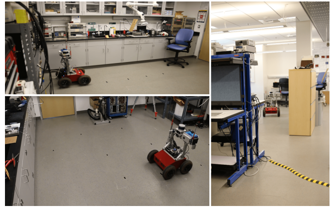
Fig. 6: Collage of experiments being carried out in the small (top left and bottom left) and large (right) laboratory environments with a ground robot equipped with a gamma camera.
